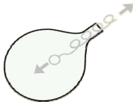
Fig. 10. During humming the sinus cavity behaves as a kind of Helmholtz resonator. The humming oscillations induce movement back and forth of the airplug in the neck of the container like a mass on a spring. This movement increases the gas exchange from the container.
